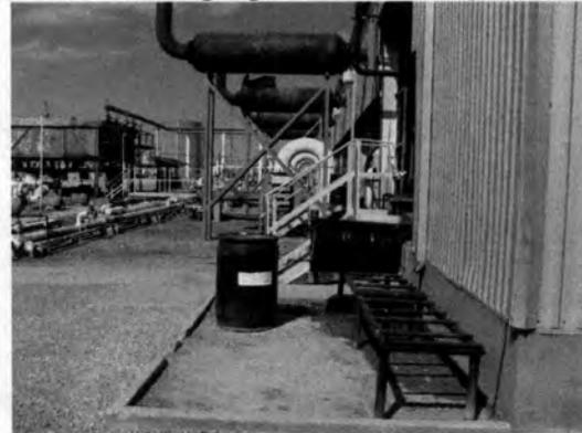
Photo 18: Improper barrel storage.
