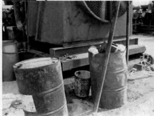
Photo 17: Improper barrel storage.
