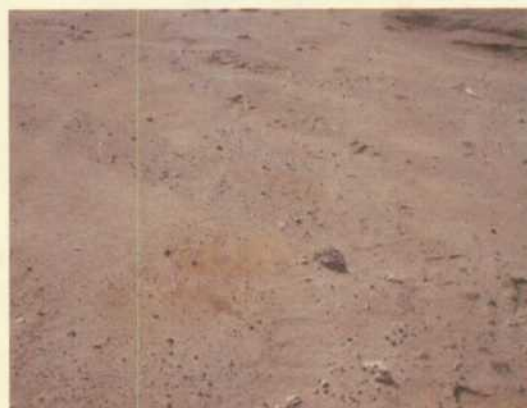
Yellow stain soil found near old chromate monitor well area 75 feet east of flare stack.
