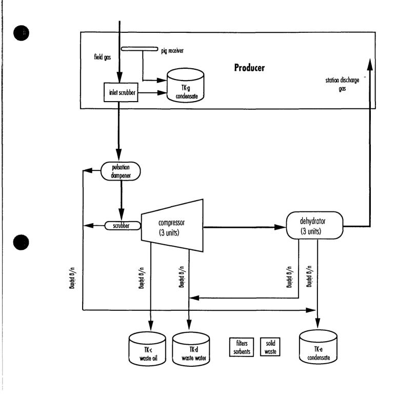
Manzanares Compressor Station Effluent and Solid Waste Production Diagram
