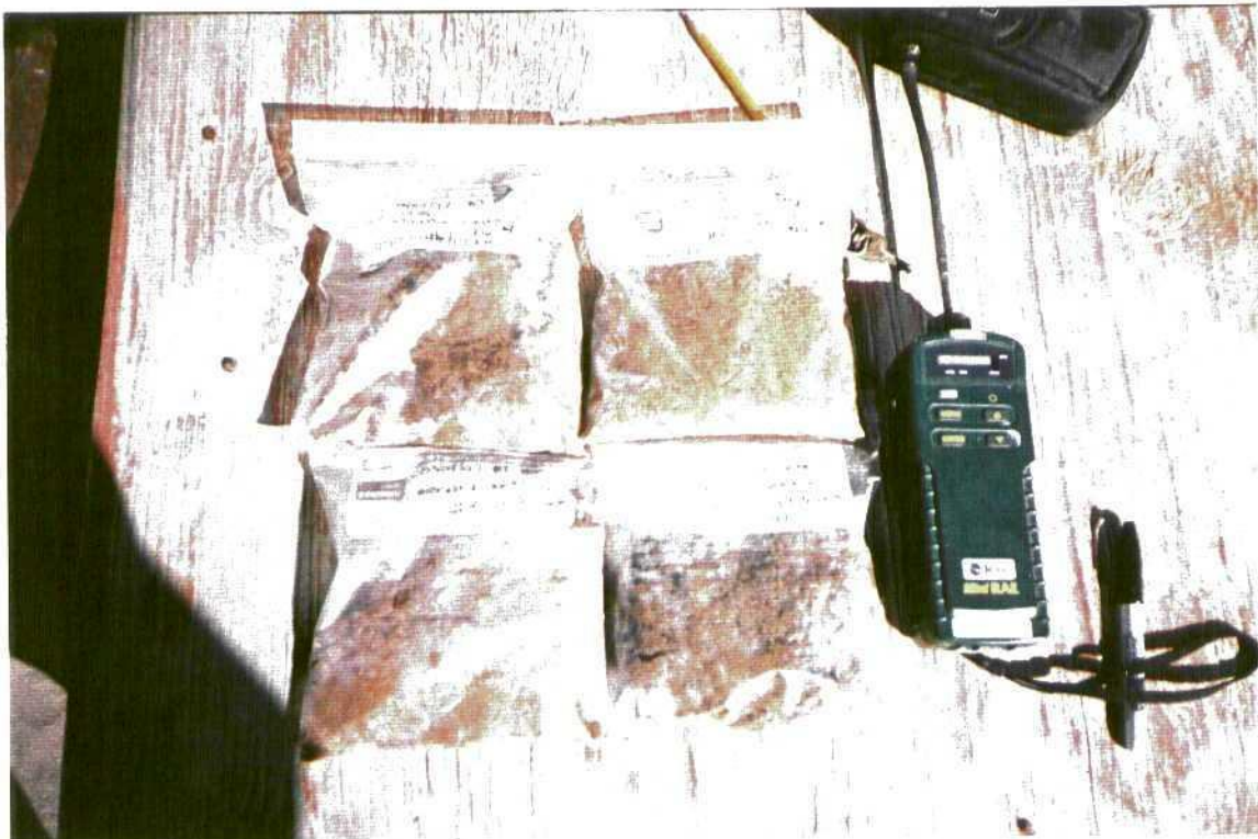
Photograph #19 Soil field screening method
