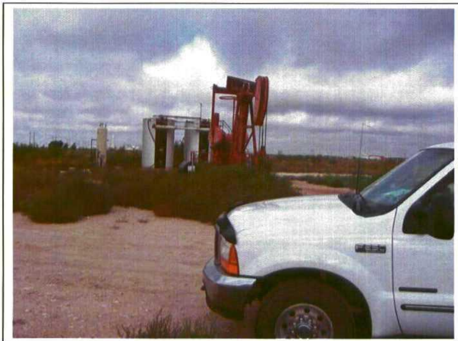
Photograph 4. Oil well pump jack and tank battery, adjacent Area 2.
