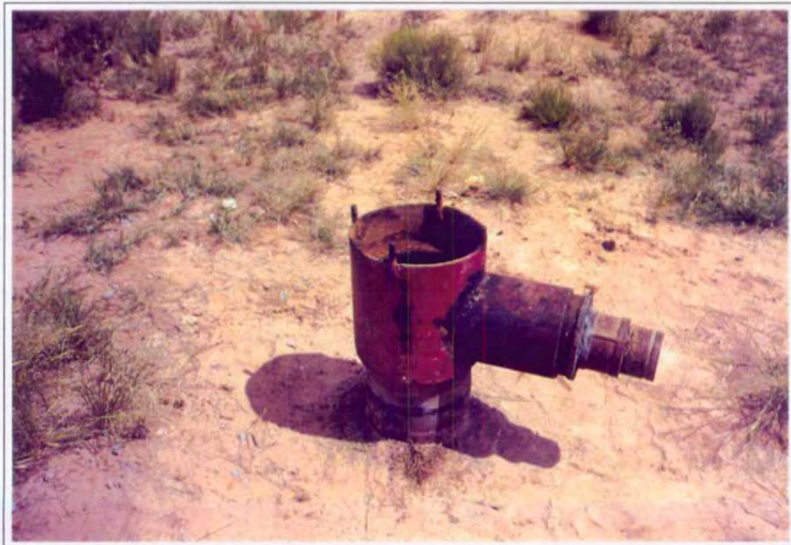
Diverter Welded to Monitor Well 6-2 Surface Casing
