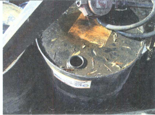
Photo 3: Bung missing on barrel.
