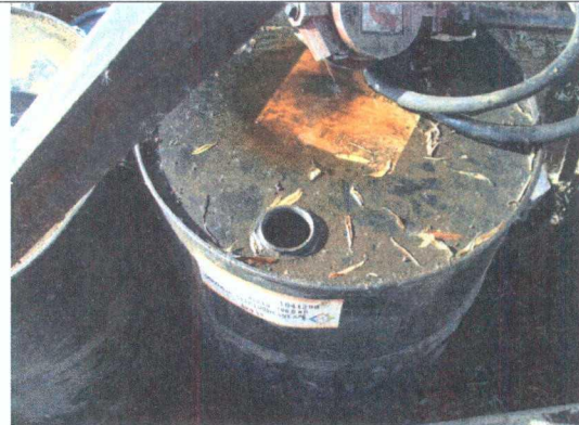
Photo 3: Bung missing on barrel.
