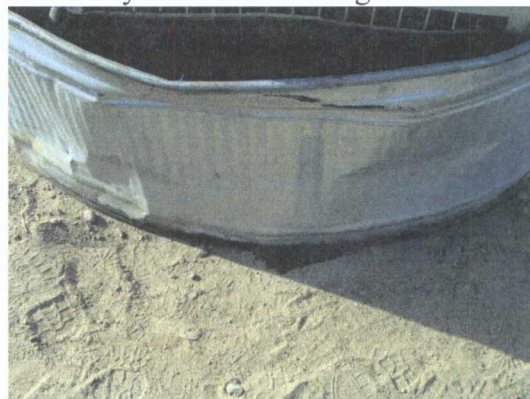
Photo 10: Secondary container with staining underneath.
