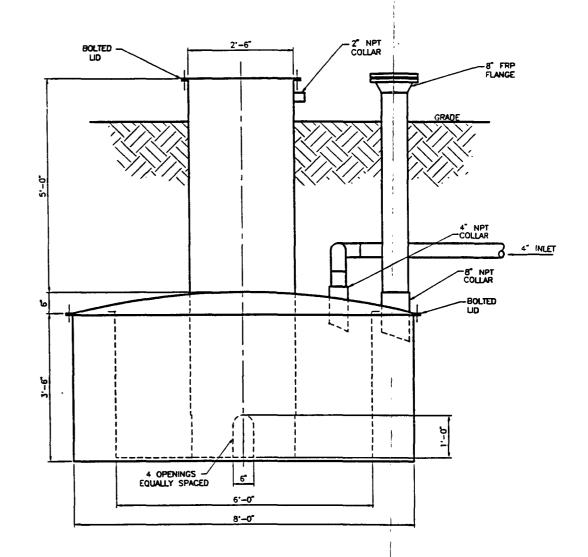
WASTE WATER SUMP ELEVATION
