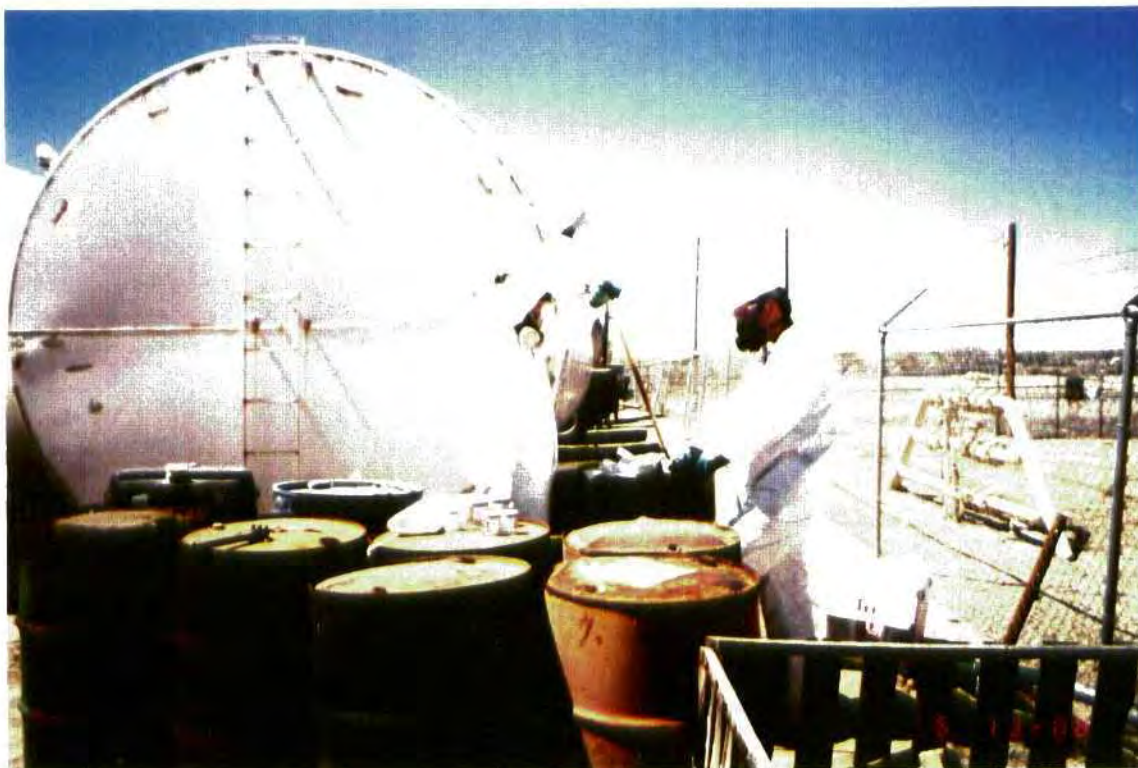
Date: 04/05/95 Picture Taken by: Mark Butler, PRC Direction Facing: W Picture Description: PRC collecting sample CDI-DRSI-10 from the drum marked as containing a scale inhibitor
