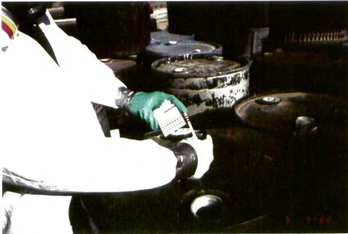
Date: 04/05/95 Picture Taken by: Luis Vega, PRC Direction Facing: NW Picture Description: pH field test of Drum 35 in the west drum storage area
