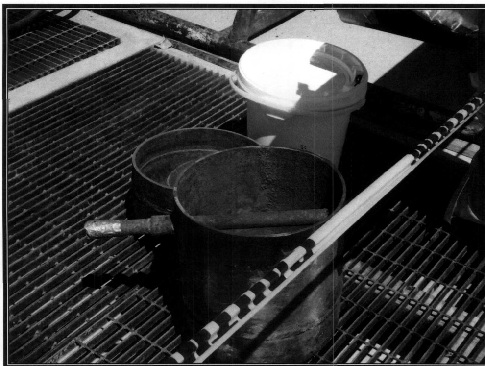
Photo 6: End Caps of Line Drip on Containment after Cutting
