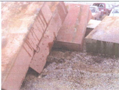
Photo 7: Over turned containments draining fluids on ground.
