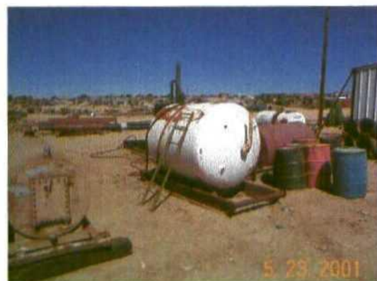
Used glycol tanks – needs containment
