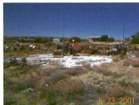
Alkali covered area sampled as hazardous material – TCLP analysis done
