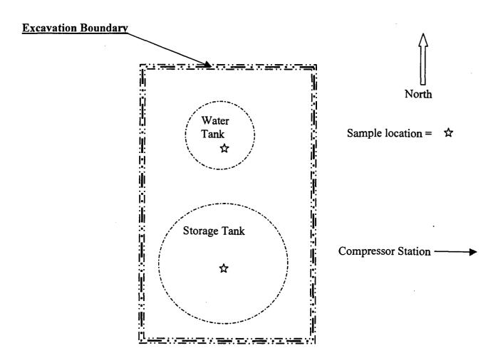
Sample from Water Tank collected at 8 feet PID field reading 0.0 ppm
