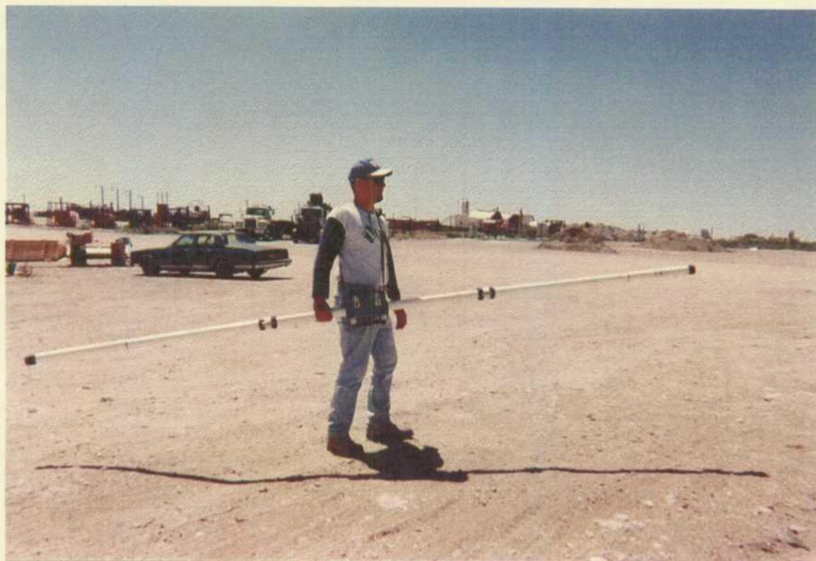
Photo Number: 7 Photographer: A. Garza Location: Rowland Trucking Company Subject: EM 31 electromagnetic survey City/County: Carlsbad State: NM Date: 04/22/98 Time: 1:30 PM Weather: Sunny
