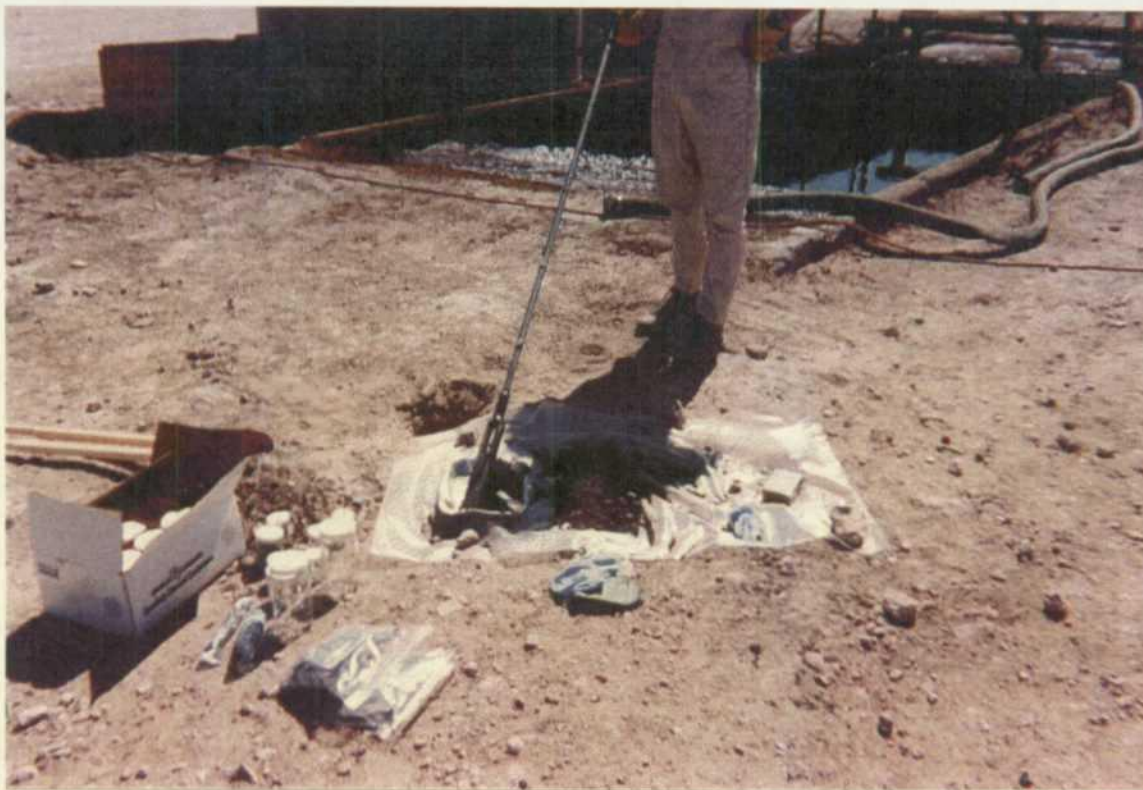
Photo Number: 17 Photographer: L. Vega Location: Rowland Trucking Company Subject: Tetra Tech personnel collecting samples RTC-SS-02A, AD, B & BD City/County: Carlsbad State: NM Date: 04/22/08 Time: 3:00 PM Weather: Sunny
