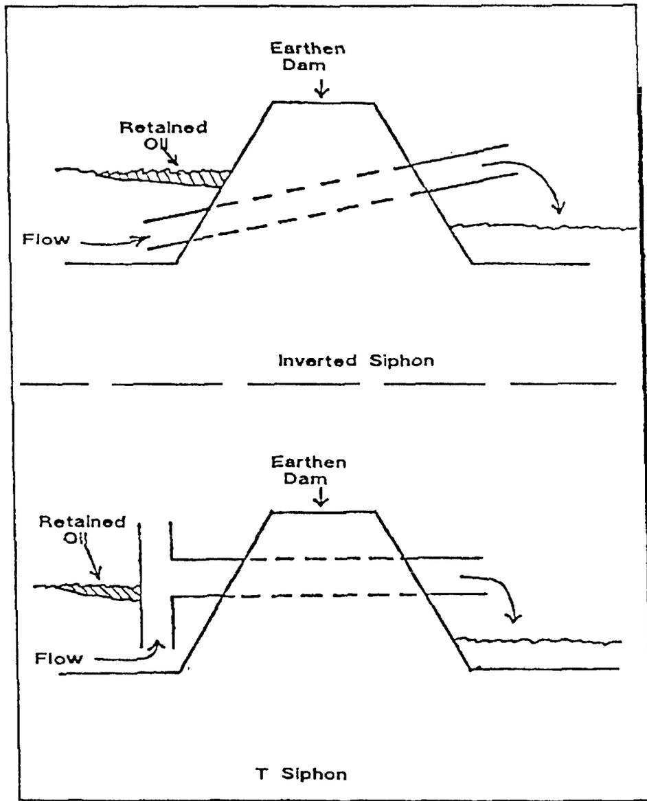
Figure D-5. Earthen Dam Construction.
