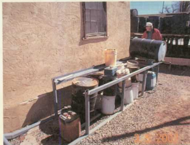
Drum Storage Area in yard of Chaco Chemical No containment.
