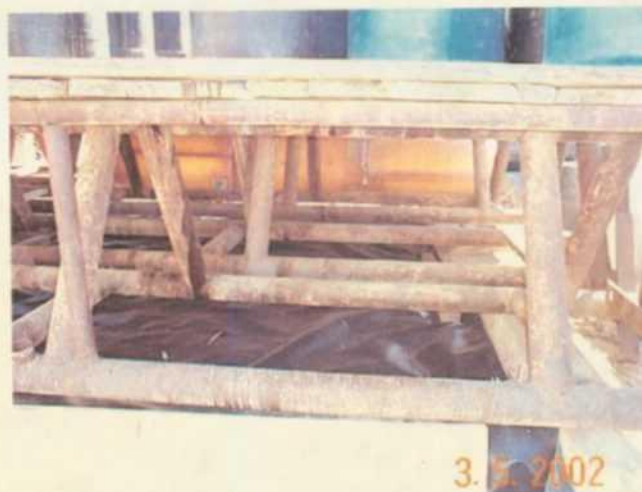
Elevated rack for chemical drum storage at Chaco Chemical. Note plastic liner beneath.
