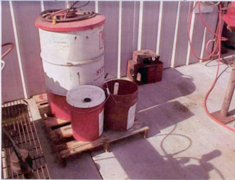
Guardian Wellhead Protection, Inc. Hobbs Service Facility Drums and buckets containing fluids without secondary containment
