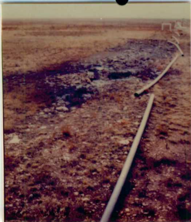
Fig. 1 Brine and oil above a leak in the pipe line
