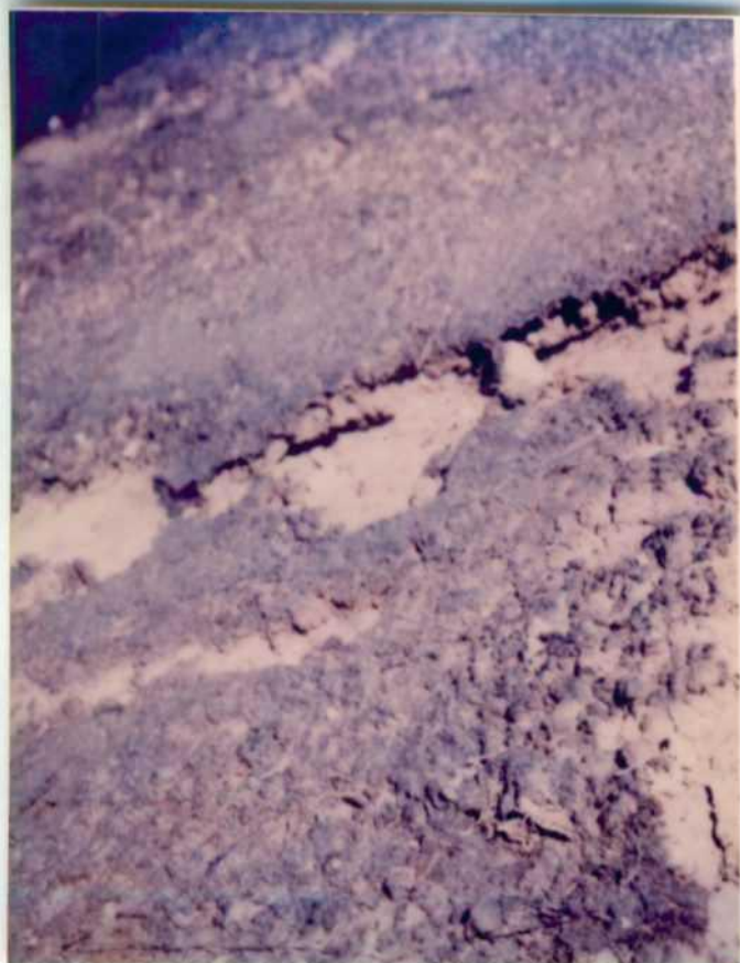
Fig. 3 Rainwater erosion of the pit wall. Surface of standing brine and oil at upper left
