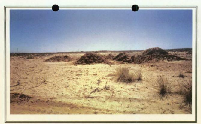
Photo 9. Existing excavation soil piles showing dark staining.
