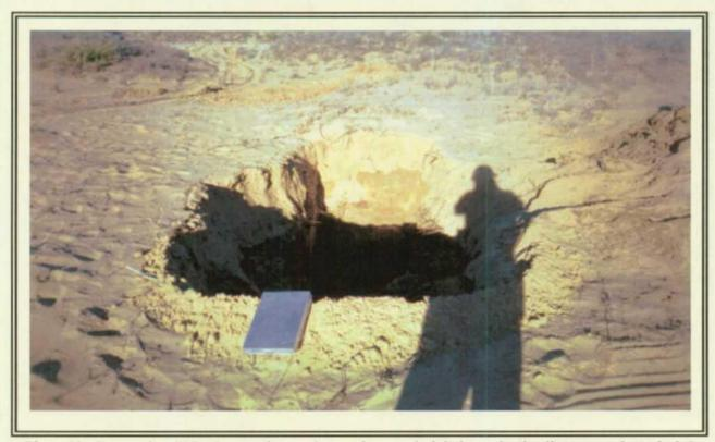
Photo 12. Excavation #15 – Loose, dry sand at surface, underlain by stained soil at approximately 2.5 feet below ground surface.
