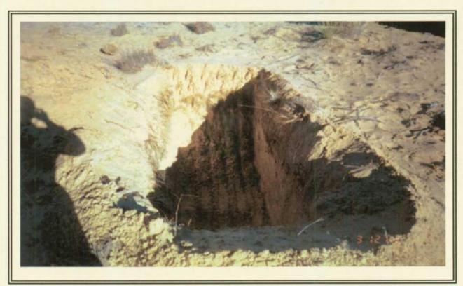
Photo 10. Excavation #7 – Stained soil evident at about 2 feet below ground surface in right side wall.
