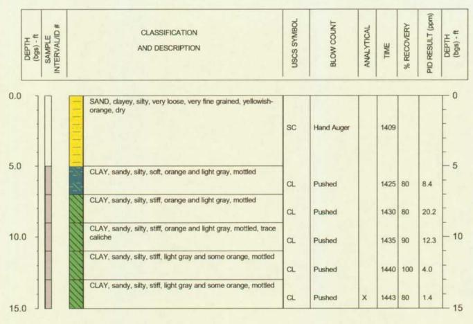
PROJECT NAME: Maxim #2690018 SOIL VAPOR BORING NO. B-9 LOCATION: Reed A, Lea County, New Mexico FIELD LOGGED BY: K.Henderson DRILLED BY: Scarborough Drilling DATE HOLE DRILLED: 3/13/02 DATE ABANDONED: 3/13/02 Not Encountered (ft) GROUNDWATER LEVEL (bgs): REMARKS: bgs = below ground surface ND=Not Detected, NS=No Sample DRILL TYPE: Air Rotary NA=Not Applicable Ford Midway 1300 (in) BORE HOLE DIAMETER: 5
