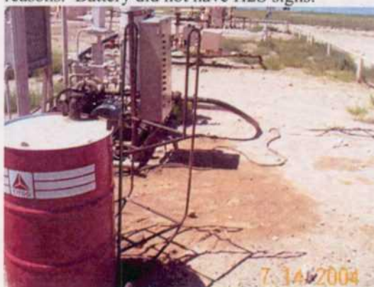
Penroc Battery State 11-23 picture shows gas line. Line was noted to be leaking and a slight H 2 S smell was noted. Did not sample for safety reasons. Battery did not have H 2 S signs.
