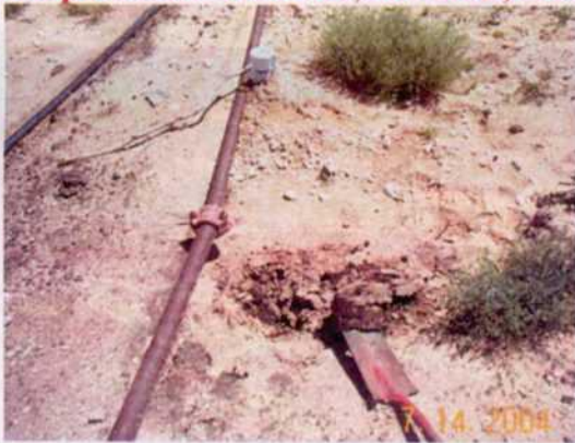
Flow lines between well #2 and 11-23 battery. Collected soil sample 6-8 inches deep found oily dirt. Collected soil sample field code # 0407141455.
