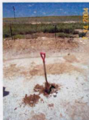
Harris State #5 site-Salt contaminated soil found east of tank inside of berm area. Collected soil sample # 0407141400 field code.
