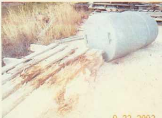
Photo 7: Drum and a wood pallet disintegrated by what looks to be caustic or spent caustic. Southwest corner of site.
