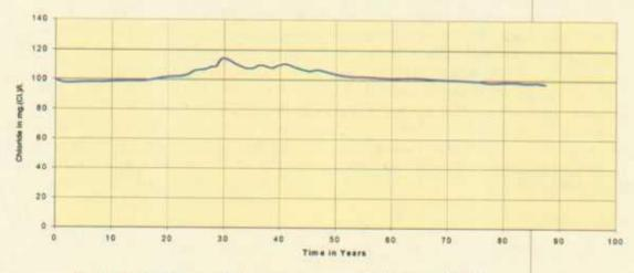
Figure 4. Chloride concentration assuming an aquifer thickness of 130 feet.
