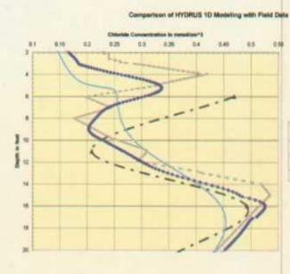
Figure 5. Predicted chloride concentrations of January 2005 simulations
