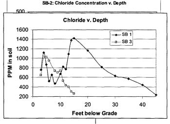
The pattern for SB-1 shown in Figure 3, which was closest to the pipeline rupture, confirms that the October 2003 release is not the first release at or near this site. An earlier release appears as chloride concentrations above 1000 ppm between 12 and 20 feet below grade and the October release appears as the high chloride between 3 and 6 feet depth. We do not believe that the chloride concentrations between 12 and 20 feet in SB-1 were caused by the 10-barrel release of June 2003.
