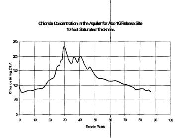
Figure 6. Ground water chloride concentrations in imaginary monitoring well.
