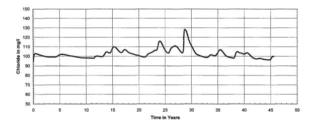
Figure1 : Chloride Concentration Observed in the Aquifer at the Down Gradient Edge of a North-South Road with a 6 inch thick Layer of 1200 ppm Caliche
