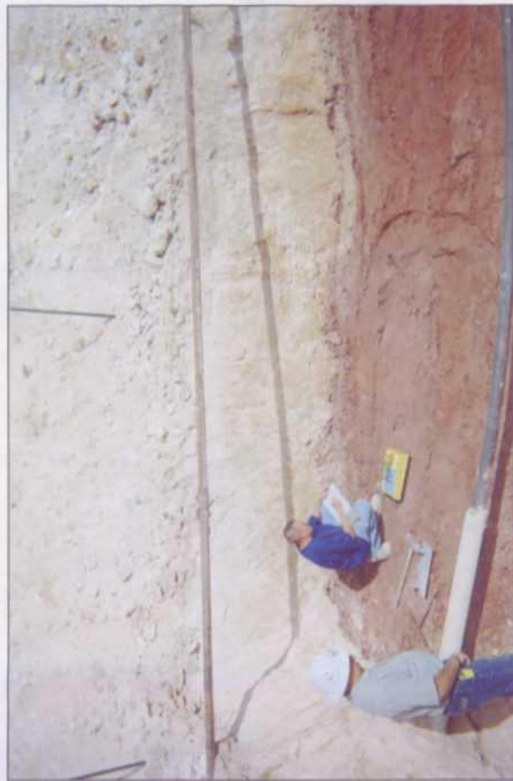
testing compacted clay at 6 ft BGS
