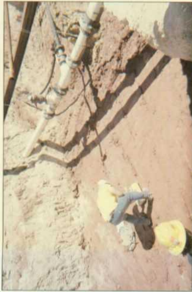
testing compacted clay at 6 ft BGS 4/21/2004
