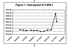
Figure 1 is a hydrograph of the E-5 monitoring well of Rice Operating Company, which is gauged quarterly. In the area of the Bertha Barber site, water levels rose more than 10 feet. Other wells in the area also showed a rise in the water table elevation, but generally less than the 10 feet observed at the E-5 Bertha Barber site.
