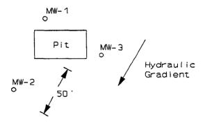
Each well will be installed by hand or power augering a 3- or 4-inch hole to a depth of approximately 3 feet below the water table. A clean one-inch-diameter PVC slotted screen will be placed to a depth of approximately 2-3 feet above the water table. The screen will be connected to a blank one-inch PVC casing.
