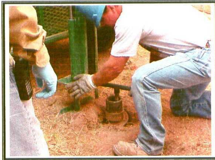
32) Hand auger sampling of second sample point 15-10-01 "B". Hand auger tool used because split spoon tool damaged.
