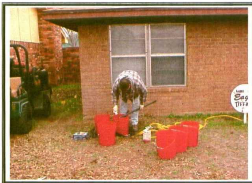
Decontamination of split spoon sampling tool
