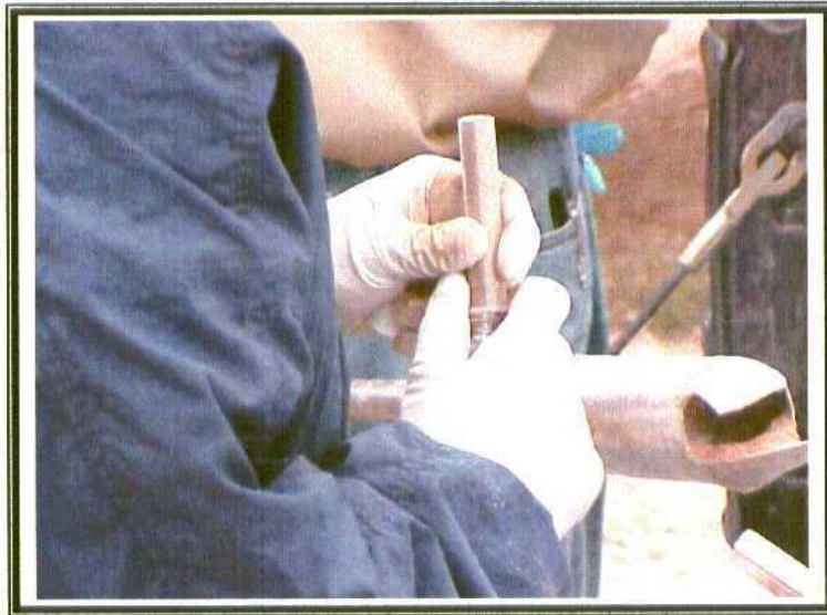
14) BBC technician filling methanol preserved sample vial at WSB-01 sample point.
