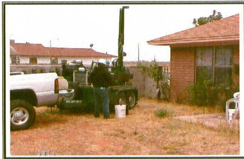
1) Portable rig setup in Rising's backyard. Sample point 13-03-01.
