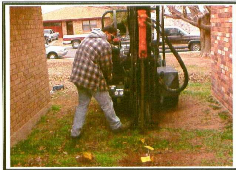
Soil Sampling – Borehole #1506-06
