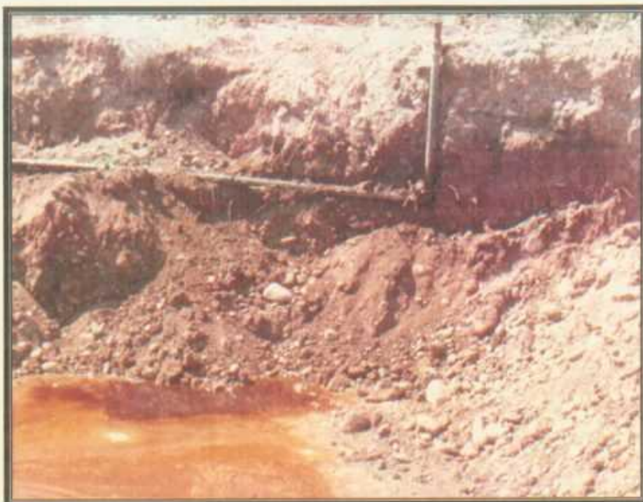
Photo 9: Additional Contamination from a Pipe Leak under the Separator
