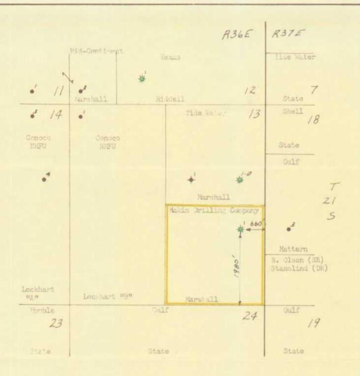
MAKIN DRILLING COMPANY APPLICATION FOR NOT- TAIDARD GAS PROBATION UNIT OF 150 ACRES, MINO S /L SECTION 13, T-115, R-36E, EDMONT GAD POOL, LEA COUNTY, NEW EXICO.
