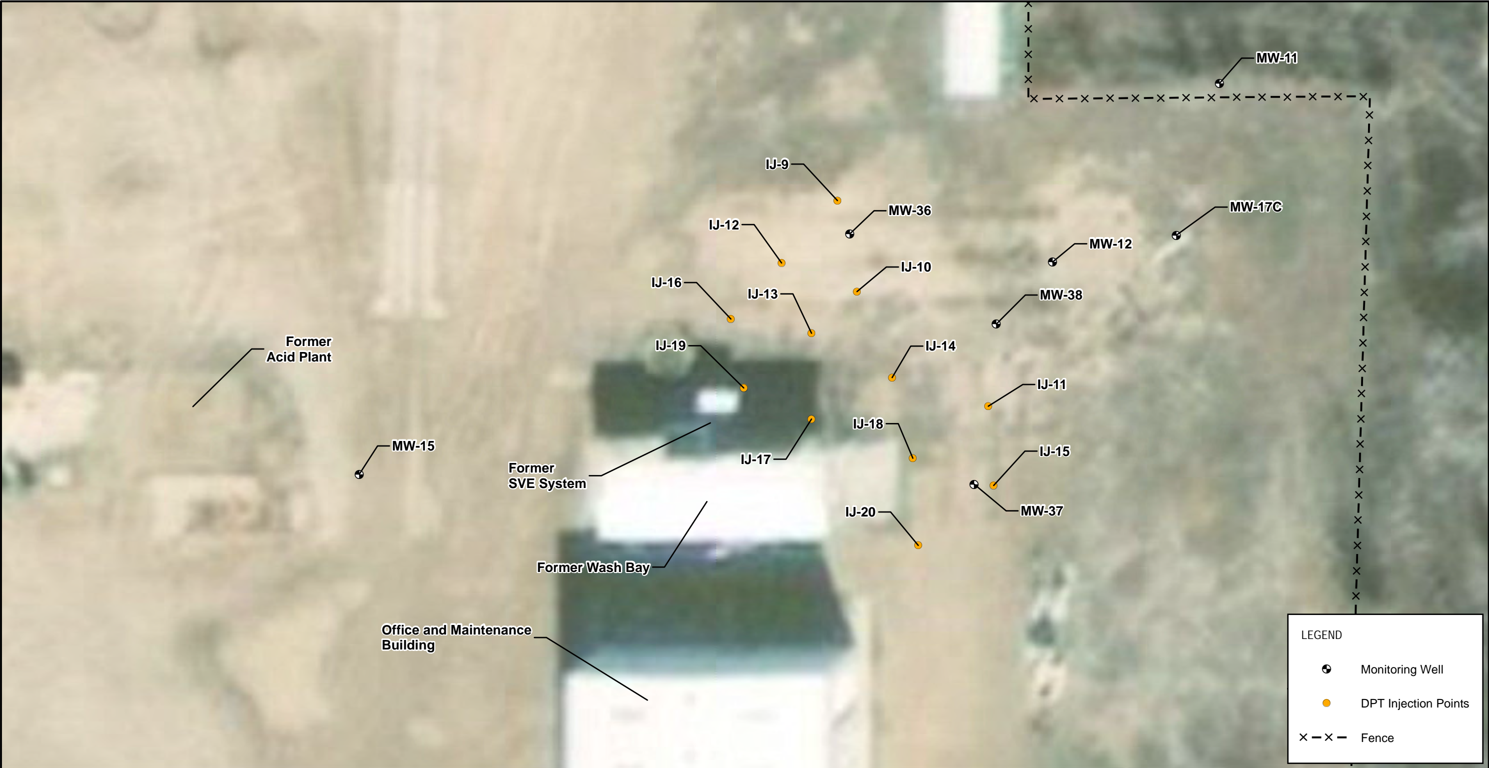
Figure 3-1. DPT Injection Locations 2019 Annual Groundwater Monitoring Report Former Dowell Schlumberger Facility Artesia, New Mexico
