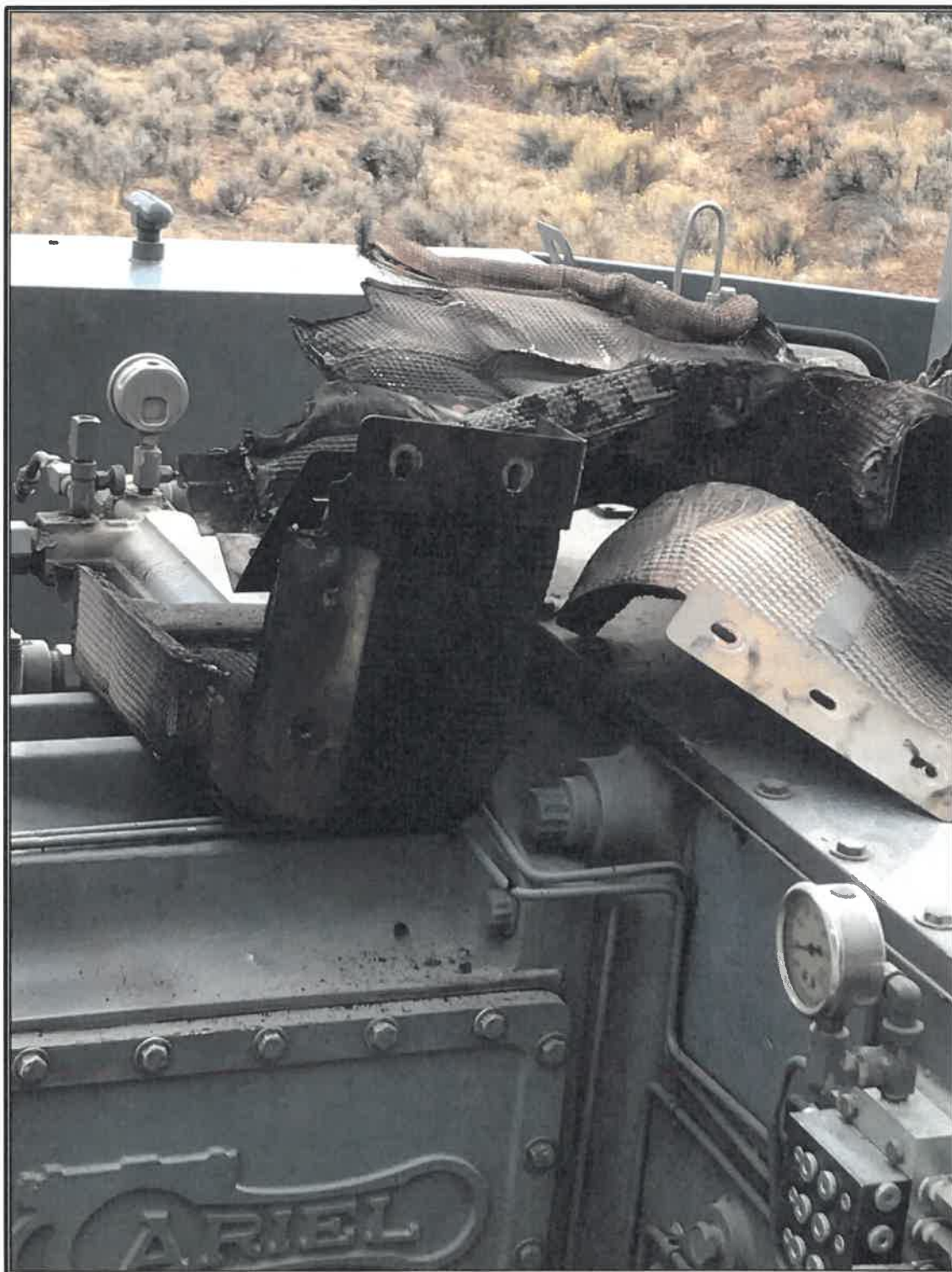
PHOTO 2: View of Damaged Insulation after Being Removed from Turbo Booster
