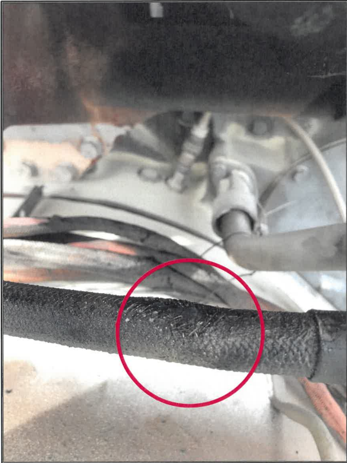
PHOTO 3: Close Up of Leaking Oil Hose
