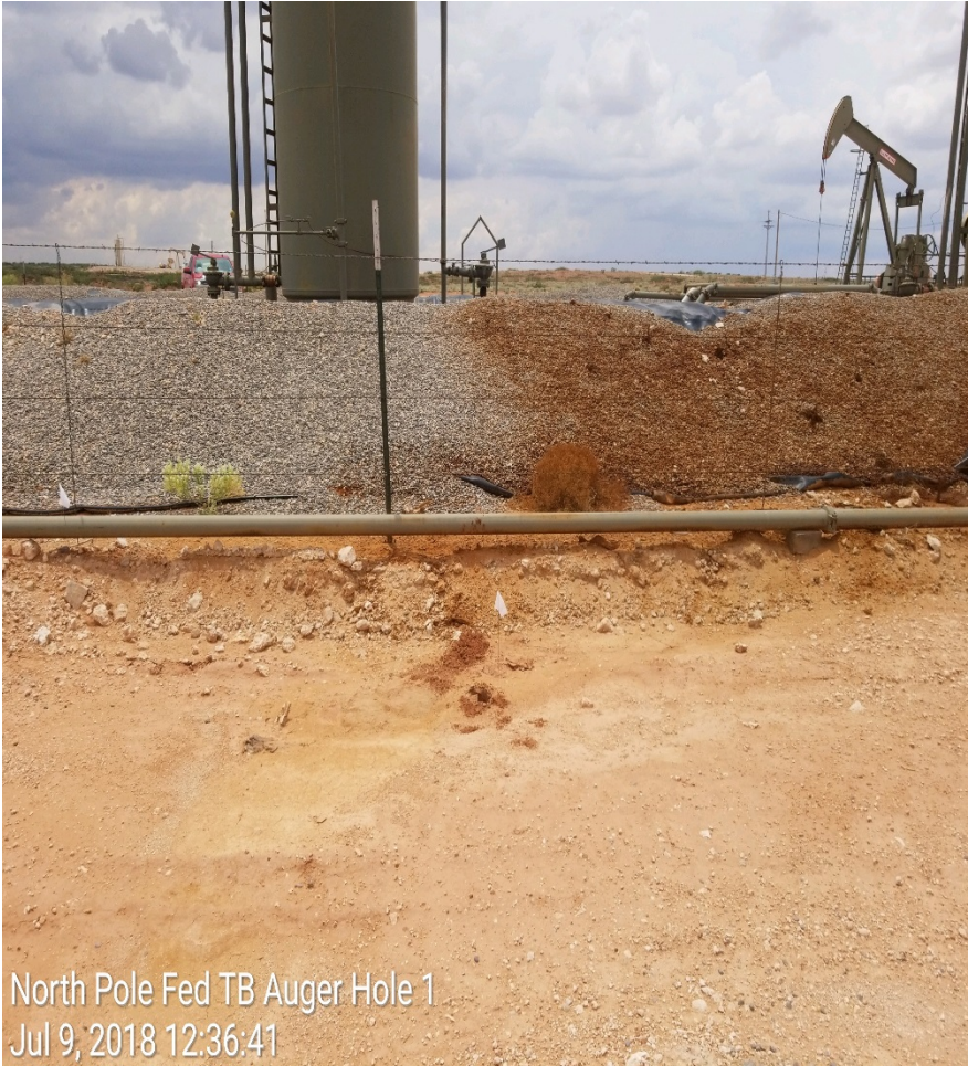
View Northeast— Origin of spill. Release caused by failed gasket on a heater treater. Area of Auger Hole-1 (flagged) middle of photograph.
