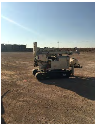
7. View of 7822DT Geoprobe rig used to advance soil borings.
