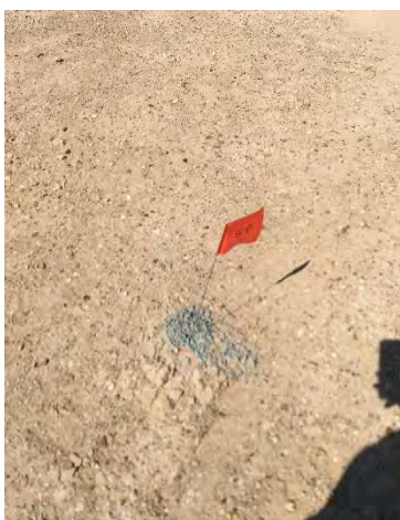
15. View of marked soil boring with bentonite plug.
