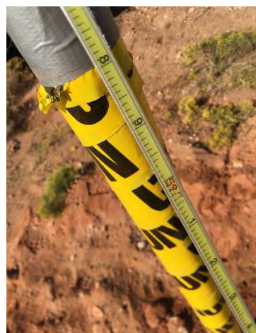
20. View of Water Level Meter showing depth of well at approximately 55'.
