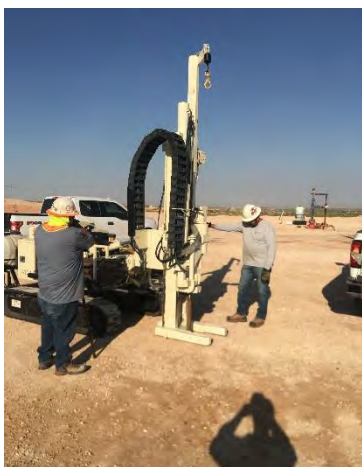
9. View of advancement of SB-01 at the caliche layer.
