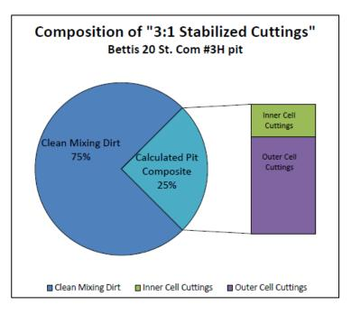
solids from the outer cell (1:3 ratio), representative of the volume of cuttings in each cell.
