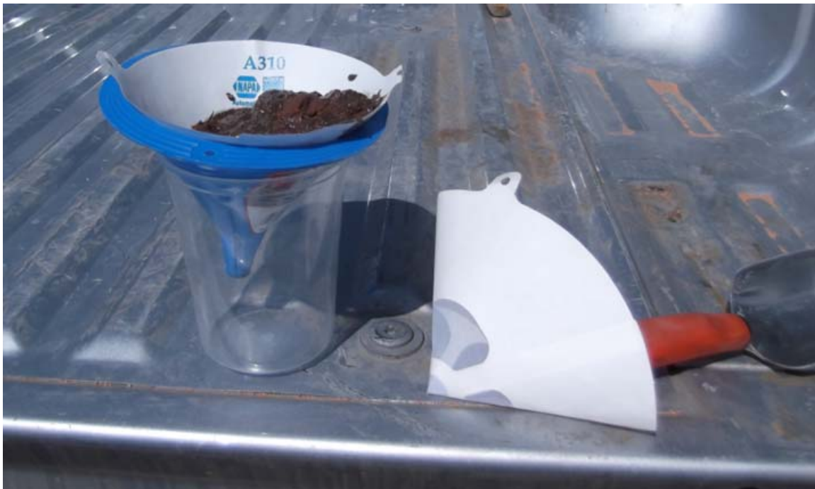
Figure 1: Paint Filter Test at Pulliam 27-P #001, March 13, 2015. The photo was taken five minutes after the completion of the test.
