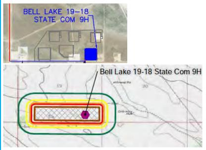
Information in this Appendix applies to reserve pits associated with proposed wells on the 9H pad (upper photo) and the two proposed pads west of the 9H. The lower image shows the setback distances described in the Siting Criteria Demonstration.
