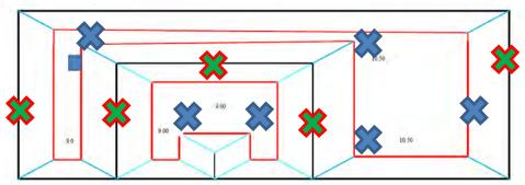
Image shows typical discrete pit sample locations (blue X) and the sub-sample locations for the "mixing dirt" (green X) composite sample to determine compliance with Table II.
