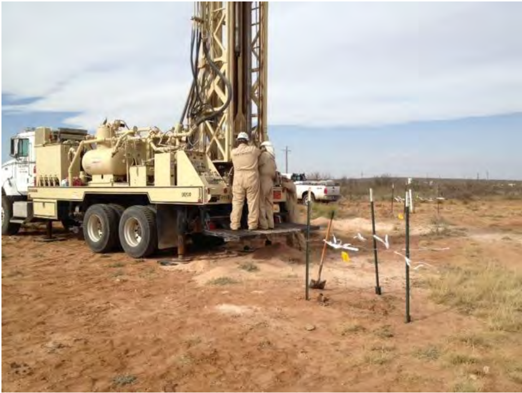
Photograph of advancement of soil bores and collection of core sample at the A-14 6" Line Historical Release Site.
