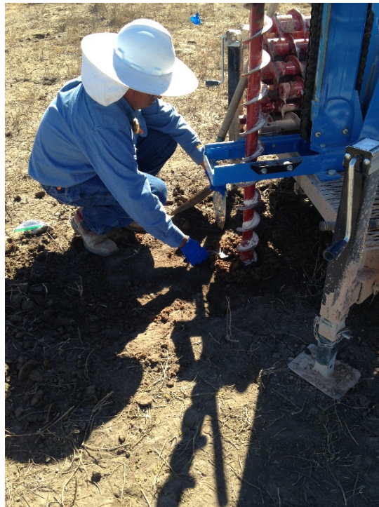
Obtaining confirmation samples from drilling bore holes
