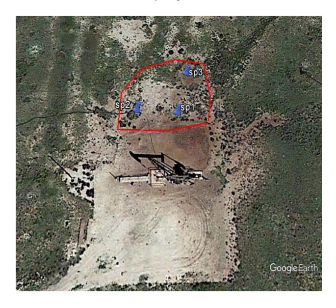
**Sample Points # 1-3** - Soil samples were obtained at 2' BGS (Bottom Hole) and confirmation samples at 12' BGS
