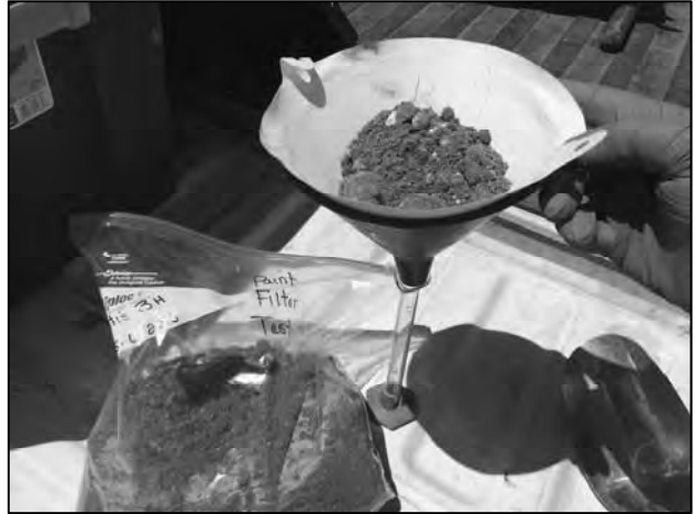
Paint filter test on stabilized cuttings 5/6/2015
