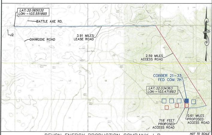
DEVON ENERGY PRODUCTION COMPANY, L.P. COBBER 21-33 FED COM 7H LOCATED 216 FT. FROM THE NORTH LINE AND 1323 FT. FROM THE EAST LINE OF SECTION 21, TOWNSHIP 26 SOUTH, RANGE 34 EAST, N.M.P.M. LEA COUNTY, STATE OF NEW MEXICO
