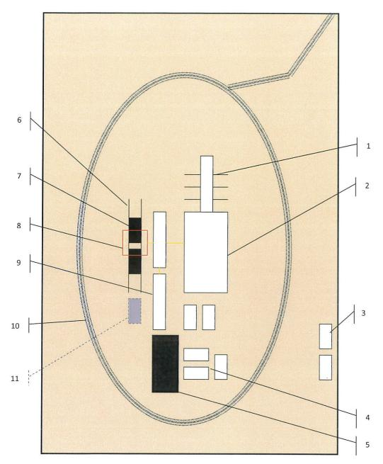
Schematic Closed Loop Drilling Rig\*
