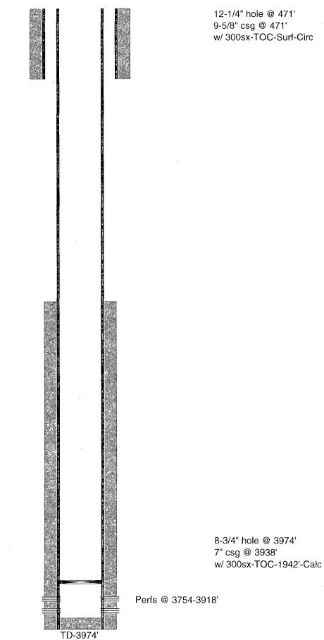
12-1/4" hole @ 471' 9-5/8" csg @ 471' w/ 300sx-TOC-Surf-Circ
