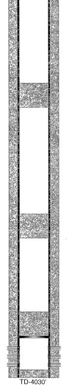
7-7/8" hole @ 4030' 5-1/2" csg @ 4029' w/ 1225sx-TOC-Surf-Circ
