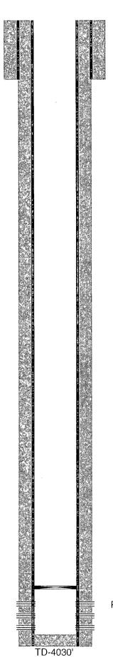
11" hole @ 336' 8-5/8" csg @ 336' w/ 225sx-TOC-Surf-Circ
