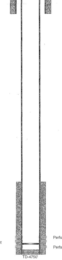
11" hole @ 315' 8-5/8" csg @ 315' w/ 200sx-TOC-Surf-Circ
