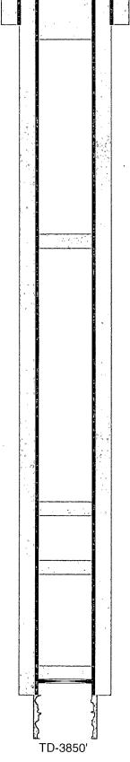
8-3/4" hole @ 3850' 7" csg @ 3699' w/ 1610sx-TOC-Surf-Circ
