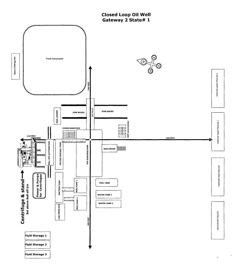
Note: The Rig and Closed System Company for this well have not been selected thus the set up shown is simply generic.
