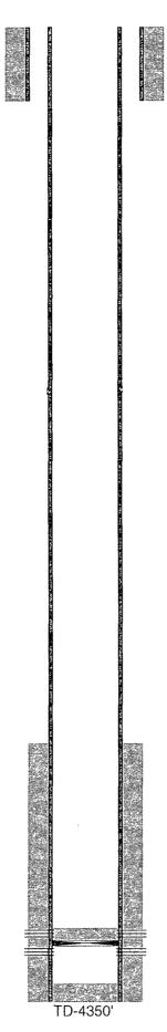
12-1/4" hole @ 382' 8-5/8" csg @ 382' w/ 200sx-TOC-Surf-Circ
