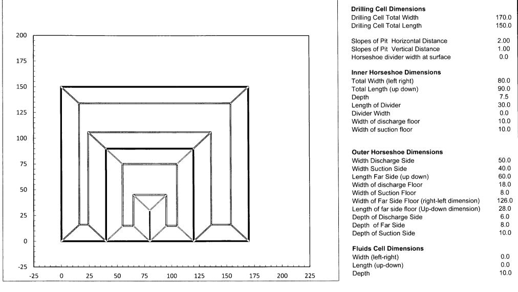
Inner Horseshoe Capacity 6011 bbl Outer Horseshoe Capacity 17701 bbl Frac Cell Capacity 0 bbl Total Capacity 23712 bbl
