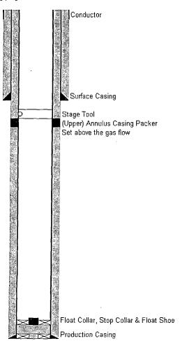
Two-Stage Cementing (Alternative for Oil / Water / Gas & Water Flow)
