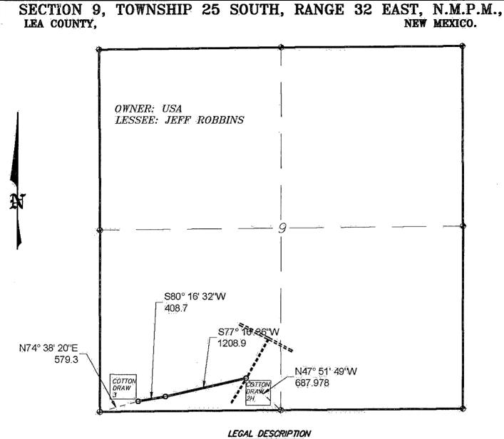
A STRIP OF LAND 30.0 FEET WIDE, L'OCATED IN SECTION 9, TOWNSHIP 25 SOUTH, RANGE 32 EAST, N.M.P.M., LEA COUNTY, NEW MEXICO AND BEING 15.0 FEET LEFT AND RIGHT OF THE ABOVE PLATTED CENTERLINE SURVEY.
